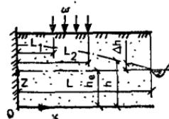
$$\bar{h}_c > 0,1 \quad \Delta h = \frac{2\omega L}{\pi^2 k_{np}} \left[ F_{11} \left( \bar{x}, \bar{L}_1, \frac{\bar{h}_c}{\gamma}, f_{0z} \right) - F_{11} \left( \bar{x}, \bar{L}_1, \frac{\bar{h}_c}{\gamma}, f_{0z} \right) \right]$$
