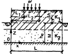
$$\Delta h = \frac{\omega L^2}{k_1 h_c^*} \cdot \frac{Z_k}{2}; \quad \left| \begin{array}{l} \sigma < 25 \\ \sigma > 25 \end{array} \right. \quad \Delta h = \frac{\omega L^2}{k_2 M} \left[ \frac{Z_k}{2} + \delta(x) \right]; \quad \delta(x) = \begin{cases} 1 & \text{при } L_1 < x < L_2, \\ 0 & \text{при } x < L_1 \text{ и } x > L_2 \end{cases}$$
