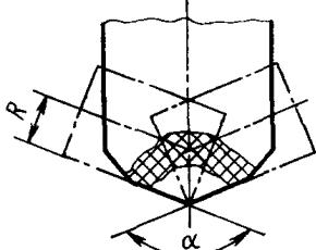
$R = 2 \text{ мм} \text{ — радиус цилиндра}$ $\alpha = 136^\circ;$ |
