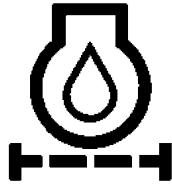
(An oil canister icon with a small horizontal line and a vertical line below it, representing a filter)      | Масляный фильтр двигателя                                                                                          | ISO 7000—1376                    |
