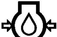
(An oil canister icon with two arrows pointing outwards from the sides, indicating pressure)                  | Давление масла в двигателе                                                                                         | ISO 7000—1374                    |
