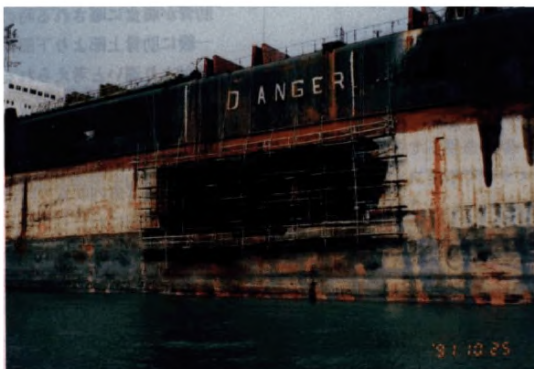
Photograph 2 Missing side shell structure (See Examples 4 and 5)
