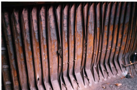
Photograph 1 Collapsed side shell frames (See Example 4)
