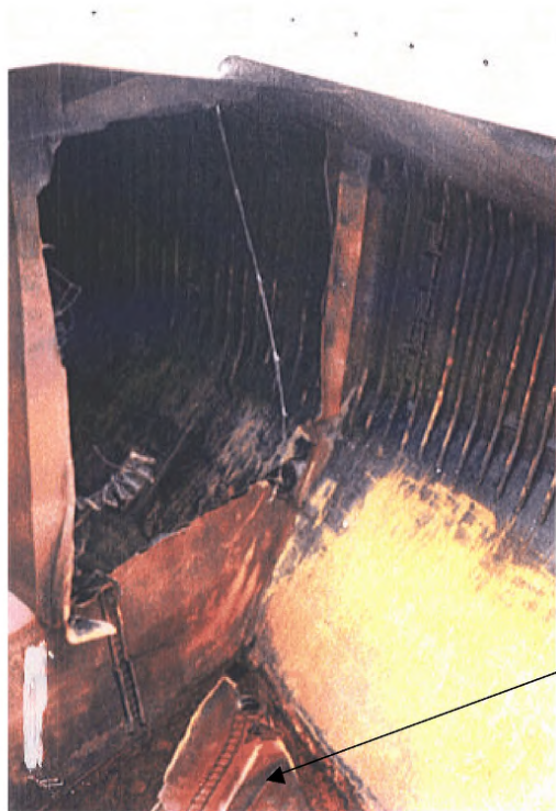
Photograph 1 Collapsed and detached transverse bulkhead
