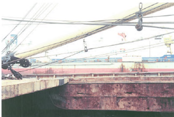
Photograph 1 Heavy corrosion of hatch coaming
