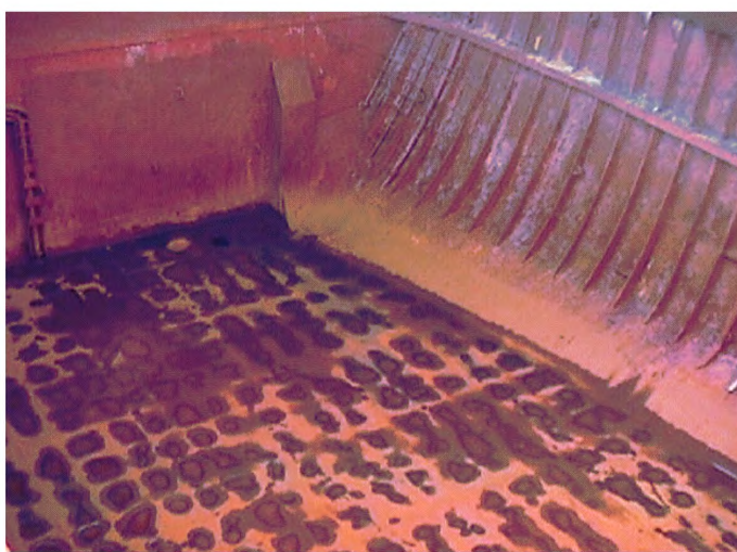
Photograph 2 Damaged inner bottom plating
