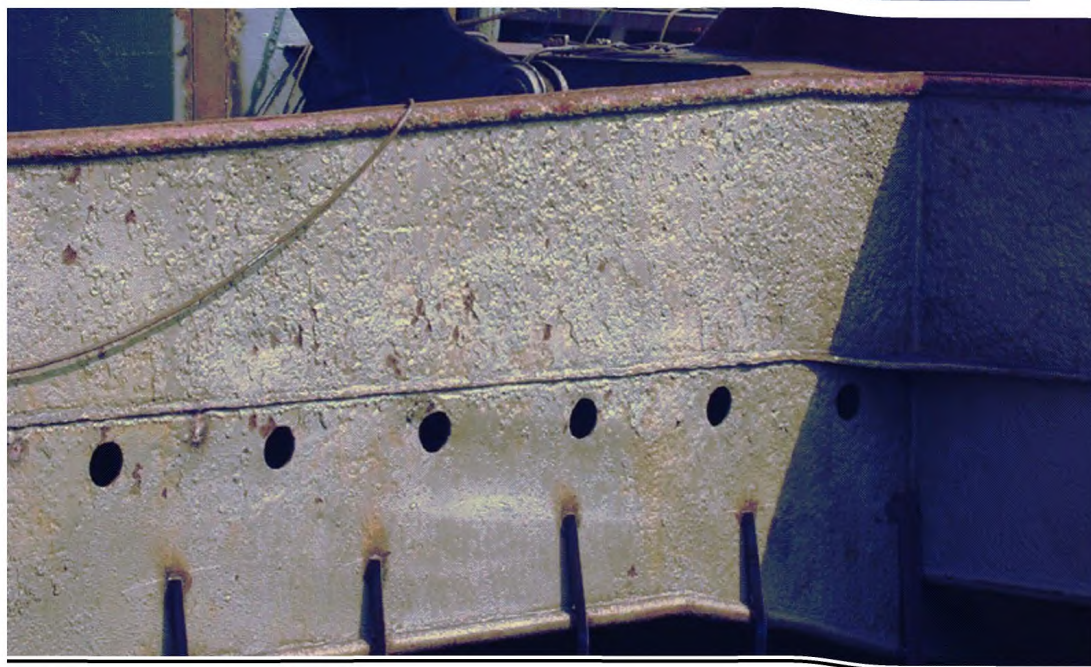
Photograph 1 Heavy corrosion of hatch coaming
