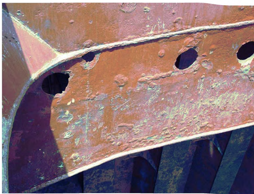
Photograph 2 Heavy corrosion of hatch coaming
