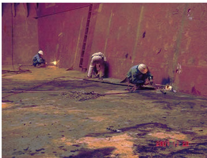
Photograph 1 Heavy corrosion affecting inner bottom plating
