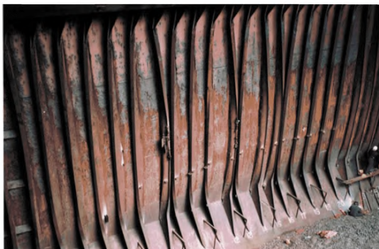
Photograph 1 Collapsed side shell frames (See Example 4)
