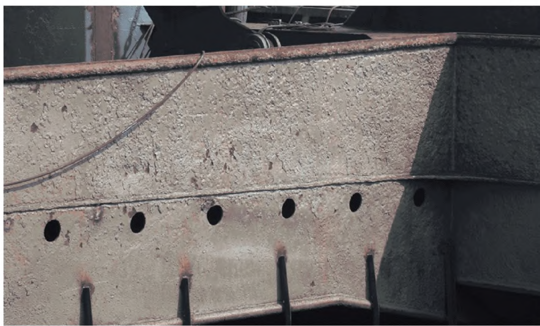
Photograph 1 Heavy corrosion of hatch coaming
