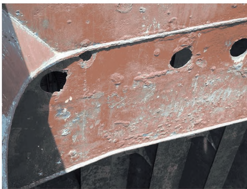
Photograph 2 Heavy corrosion of hatch coaming
