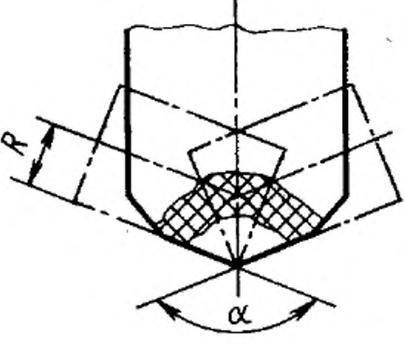
$R = 2 \text{ мм} \text{ — радиус цилиндра}$ $\alpha = 136^\circ$  |
