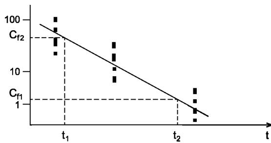
$$k_2 = \frac{\ln(C_{f1}/C_{f2})}{t_2 - t_1}.$$
