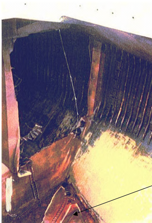
Photograph 1 Collapsed and detached transverse bulkhead
