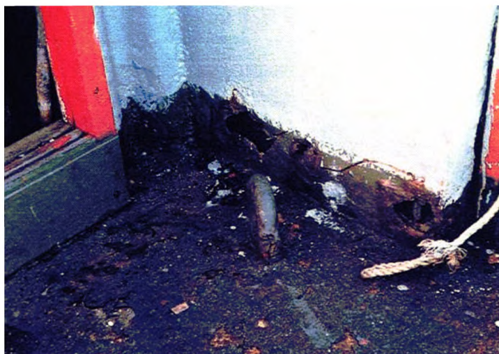
Photograph 1 Corroded accommodation house side structure
