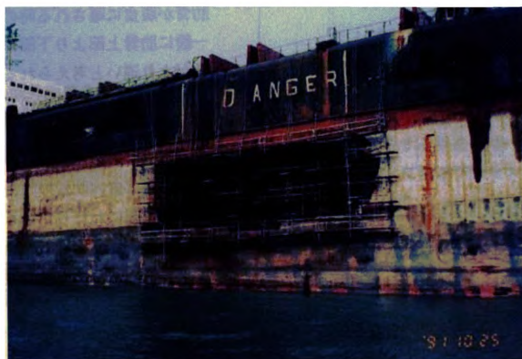
Photograph 2 Missing side shell structure (See Examples 4 and 5)
