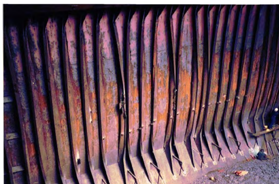
Photograph 1 Collapsed side shell frames (See Example 4)
