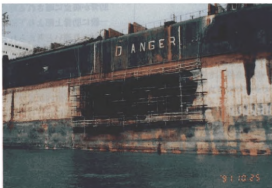
Photograph 2 Missing side shell structure (See Examples 4 and 5)
